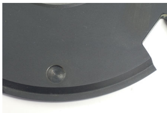
Fig. 4.1: Example of a balanced bore
