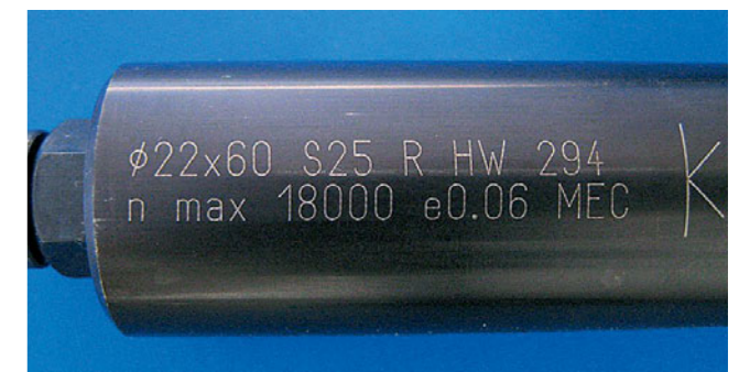
Fig. 5: Safety as a quality feature: Marking of the tool shank according to EN 847
