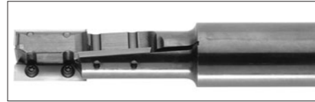
Fig. 6: Shear angle as a quality feature: Router cutter with reversible tips and small diameter
