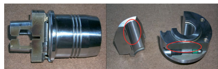
Figure 4: Layout of a hydraulic chuck
